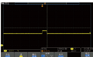
D/D Converter Surge Testing
